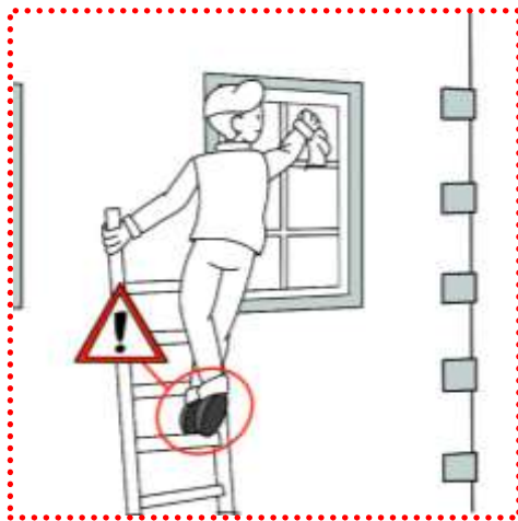
Figure 69: Bad example of overreaching and not maintaining 3 points of contact
