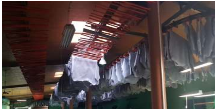
Figure 124: Overhead conveyors are often used for hang drying and transporting crust leather around tannery departments
