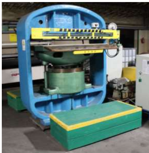
Figure 44: Reconditioned platen embossing machine to meet the present safety requirements
