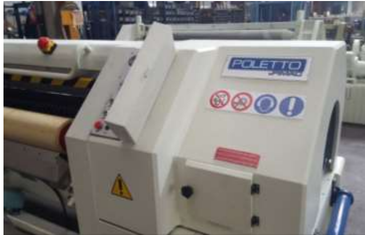
Figure 128: Fleshing machine with warning, mandatory and precautionary signs
