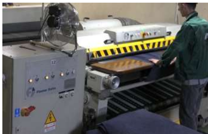
Figure 39:7 Buffing machines tend to produce excessive noise. In the picture, we can see a model with active safety device and emergency switch off button
