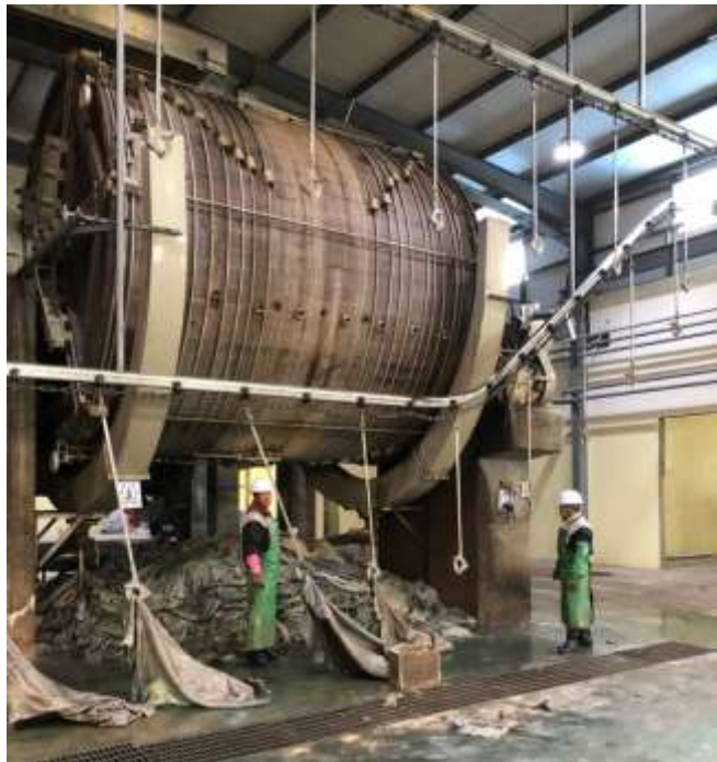
Figure 125: An overhead conveyor chain for transport of limed hides to fleshing machine
