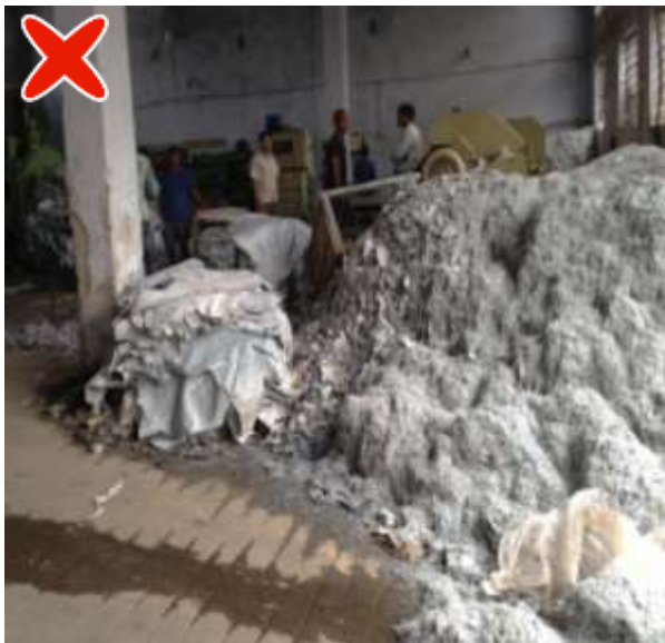
Figure 76: Piled up shavings not only pose a fire risk but also take up valuable production space
