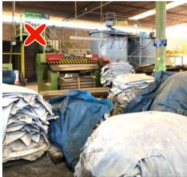
Figure 81: Bad work organization. Not enough space allowed for passing
