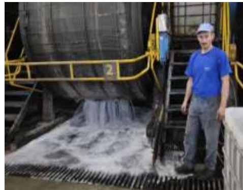
Figure 10: Exposure to chemicals by draining a retanning drum
