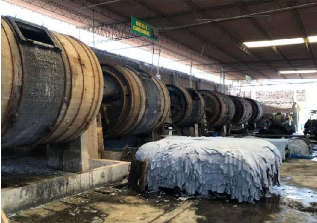
Figure 51: Tanning drums without emergency off switches nor active or passive safety guards. Manual chemical feeding and open float discharge
