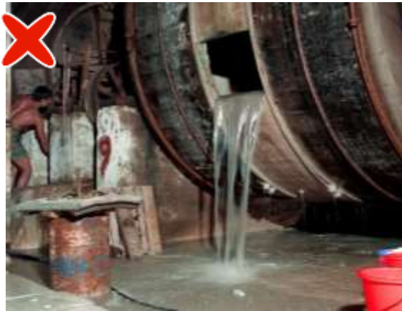
Figure 12: Uncontrolled float discharge
