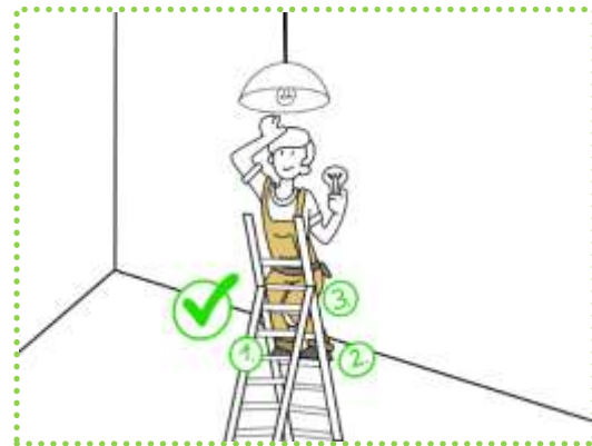
Figure 72: Maintaining 3 points of contact rule, when using both hands for work
