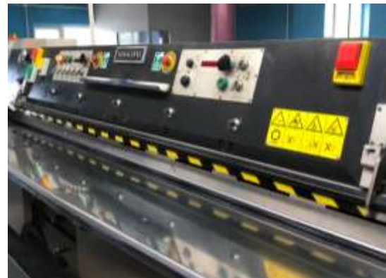
Figure 46: Active safety device on splitting machine with affixed warning signs and emergency of buttons
