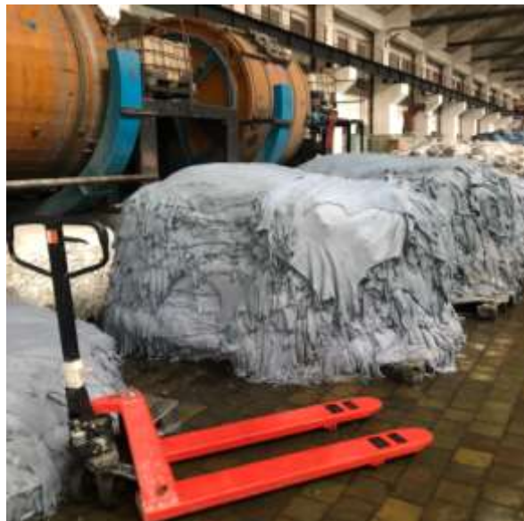
Figure 78: Using hand pallet trucks facilitate transport and save workers' from carrying heavy loads
