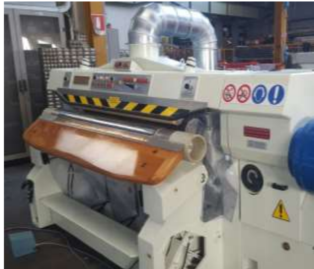
Figure 33: Dry shaving machine with exhaust system
