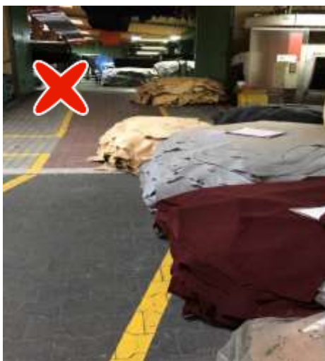
Figure 82: Obstructed access routes
