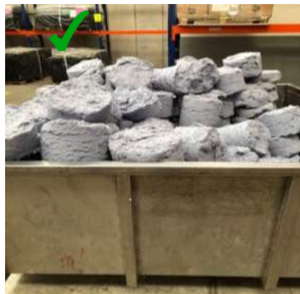
Figure 77: Shavings are readily removed from the workplace by conveyor belt, compacted and safely stored
