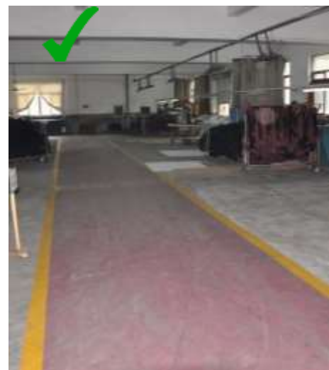
Figure 83: Marked access routes free from obstruction
