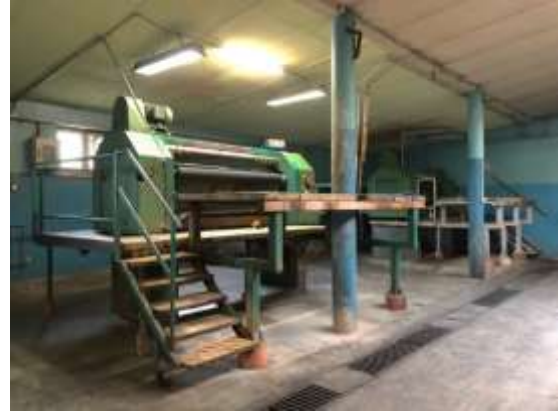
Figure 45: Fleshing m/c sitting to facilitate work, maintenance and waste removal
