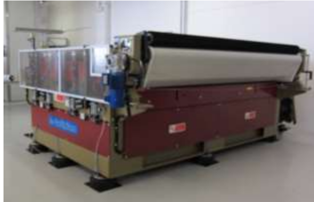
Figure 61: Vibrating staking m/c with multiple noise and vibration-dampening feet
