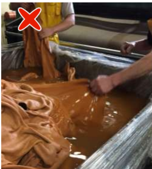
Figure 102: It is recommended to use appropriate gloves and apron
