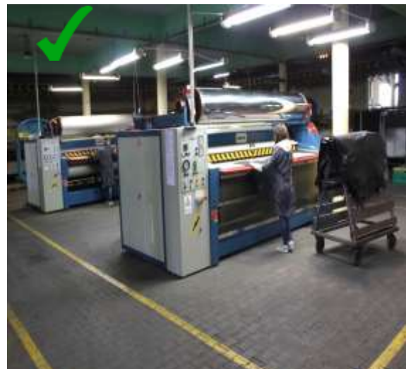
Figure 84: Sufficient space around machinery with even flooring and clearly marked passages
