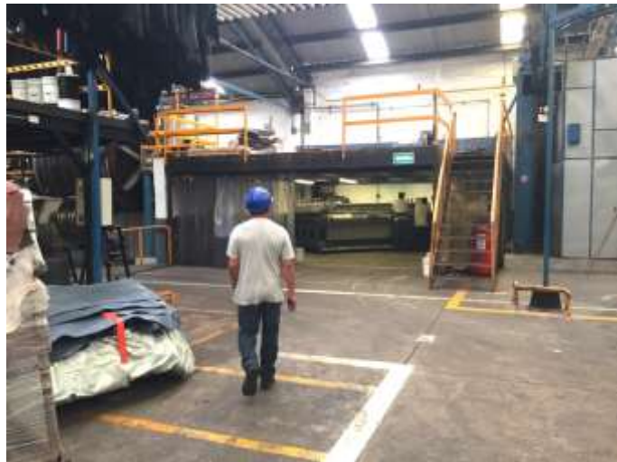
Figure 119: Make sure the traffic area is safely designed and separates pedestrians from vehicles
