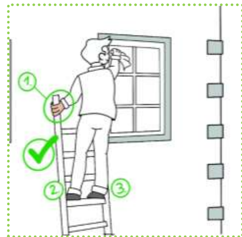
Figure 70: Good example. Work within reach and maintaining 3 points of contact
