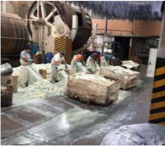
Figure 112: Workers performing "traditional" scudding operation. Well selected, adequate and comfortable PPE is key!
