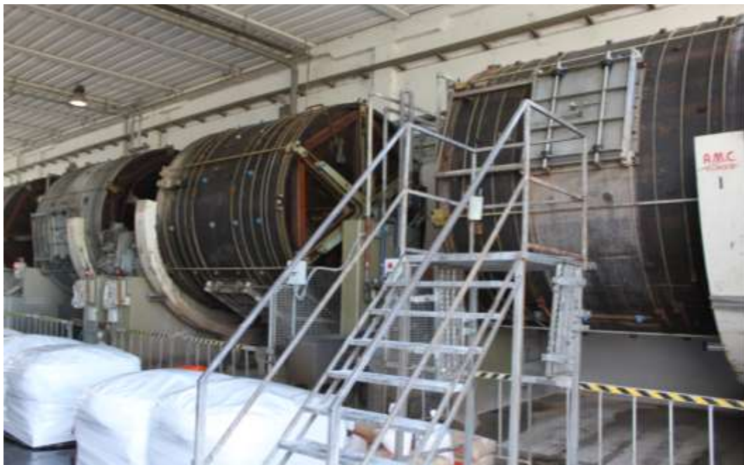
Figure 52: Tanning drums protected with active and passive safety devices, with automatic dosing (liquids) system, emergency off switches and gutters for closed discharge system
