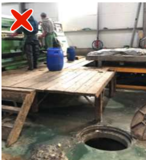
Figure 79: Open wells/lids lead to an accidents
