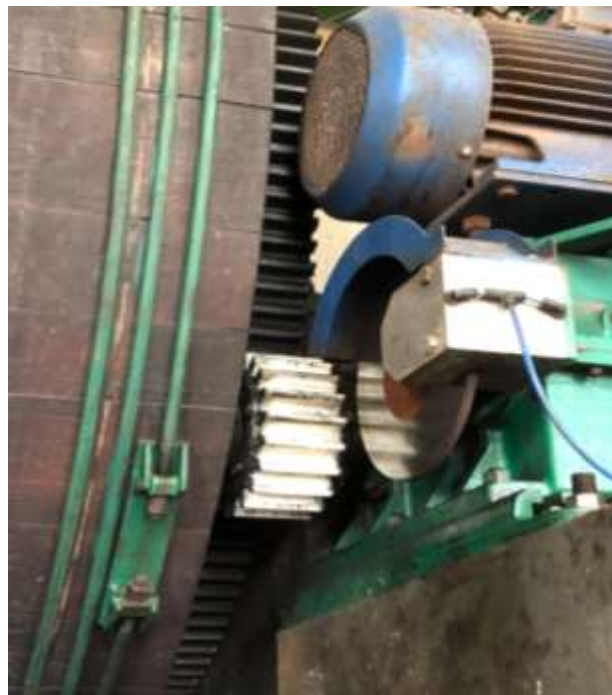
Figure 62: Low noise nylon pinion on drum drive
