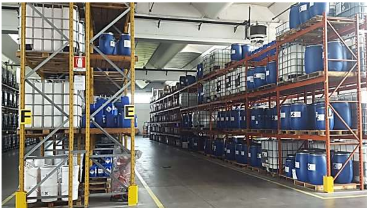
Figure 284: Proper storage lay-out and structure of a chemical store
