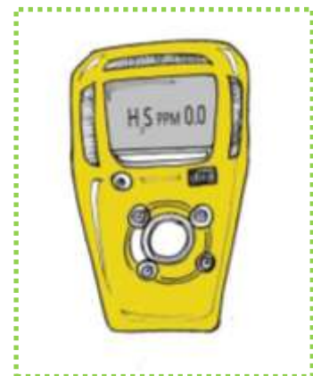
Figure 363: Use personal H_2S gas detector
