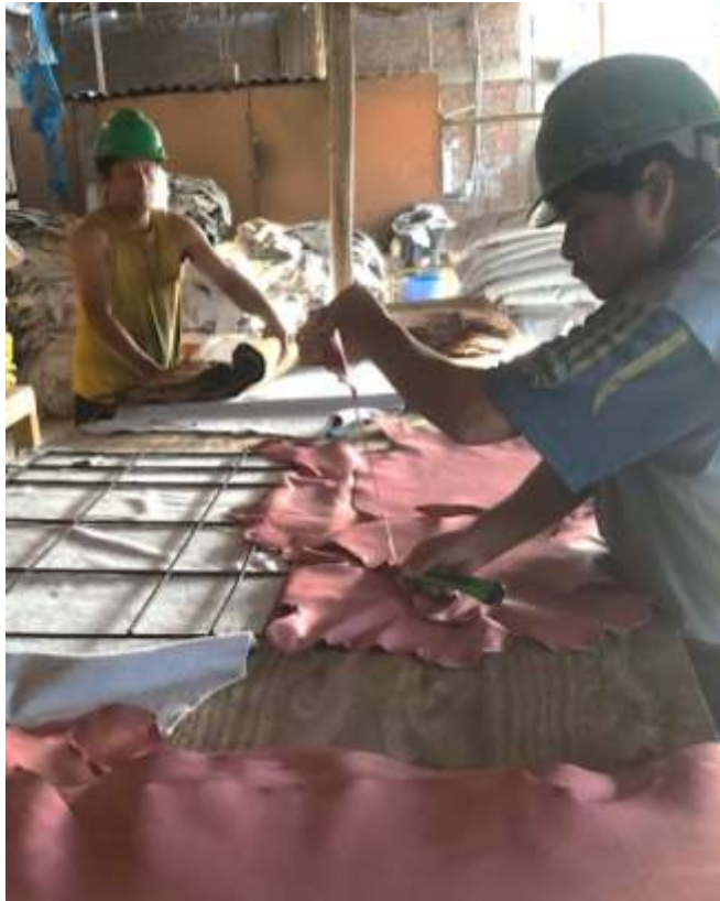
Figure 105: Leather trimming is a common operation in tanneries. The cut should be performed away from the body
