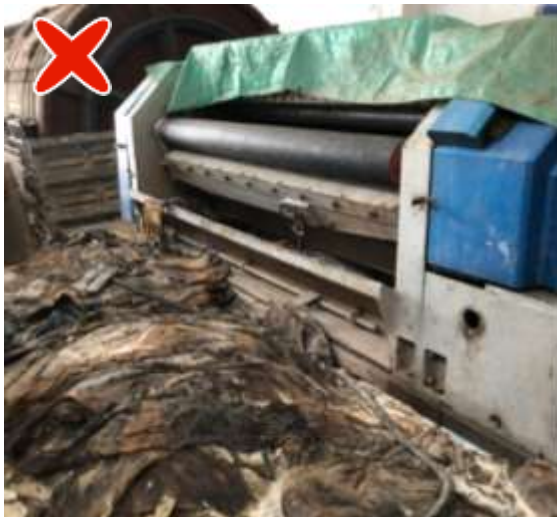
Figure 84: Dirty work area with insufficient space around the machine can be a cause of an accident
