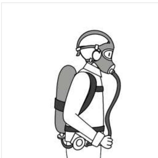
Figure 8: Self contained breathing apparatus
